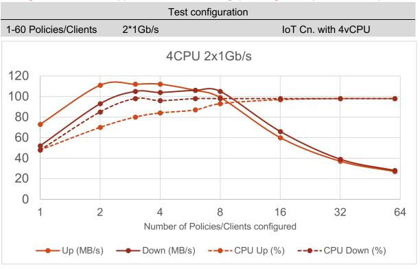
This arrangement can be used with even more Policies/Clients (8-12) and with throughputs of up to 0.9Gb/s which is the maximum expected from a 1Gbe NIC. This might for instance be a good way to support a site that has many local devices of several different types (each using their own Policy/Client), which all require isolation from the internet.
