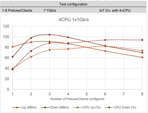
This arrangement can be used with more Policies/Clients (4-6) and where throughputs of up to 0.7Gb/s suffice. This might for instance be a good way to support a small remote office where minimal disruption to the existing network is required but where users, printers and IoT devices should be handled separately.
